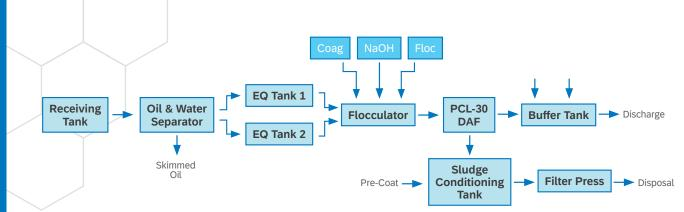
The mining truck axle facility uses various machine oils and lubricants in the manufacturing process. As with many industrial manufacturers, a substantial volume of wastewater is generated from equipment wash-down and production floor sanitation. A large volume also comes from cooling water.
